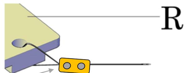
Use a metal clamp to lock the steel cable
